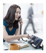
The ShoreTel BB424 gives operators 24 programmable buttons and four page keys, to handle up to 96 lines on a single box or distributed over two.
